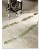
is still running, press against the knee lifter to widen your stitch to a 9mm zigzag. Release pressure to gradually return to a straight stitch for a tapered finish. Don't want a 9mm stitch? You can easily control the maximum width of the stitch setting in the machine's set mode. This advanced control opens up amazing new possibilities for creation expression with free motion quilting, thread painting, raw edge appliqué, free motion monogramming, and more.
