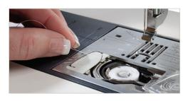
through when you first thread the machine. Slip the bobbin thread in the cover plate guide; the built in cutting blades trim the tail to the correct length for a super-clean start to your stitching line. After the initial threading, the auto-thread cutter takes care of trimming and re-setting the tails each time.
